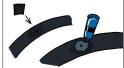
Sand the area around the puncture. Apply a **thin** layer of glue around the puncture (larger than the size of the patch) and let it dry completely.
