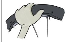
Use the heel of your hand to work the tire back on the rim, starting at the valve. If you use levers for this, careful not to puncture the tube!
