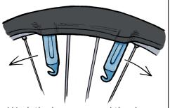
Work the levers around the rim until you've completely removed the tire from one side of the rim.
