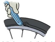
Hook the lever under the tire bead closest to you. Try not to pinch the tube with the levers.
